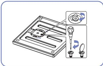
Fasten the screw tightly (using a screwdriver or coin) into the bottom of the stand base.
