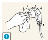
Remove foreign substances such as dust around the plug pins and power socket with a dry cloth.
