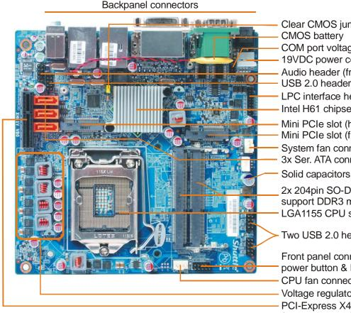
Clear CMOS jumper CMOS battery COM port voltage jumper 19VDC power connector Audio header (front) USB 2.0 header (front) LPC interface header Intel H61 chipset Mini PCIe slot (half size) Mini PCIe slot (full size)
