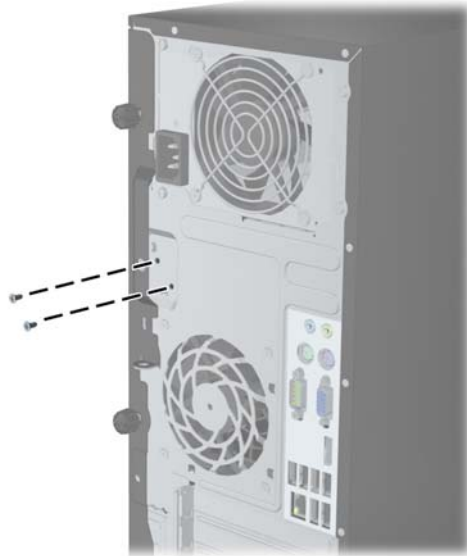
Figure C-2 Removing the Smart Cover Lock Screws from the Microtower
