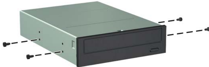
Figure 4-22 Installing Guide Screws in the Optical Drive
