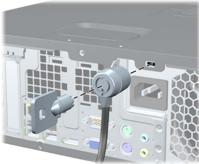
Figure 4-40 Installing a Cable Lock
