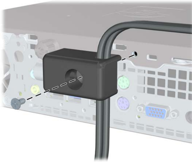
Figure 5-32 Attaching the Lock to the Chassis
