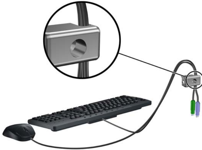
Figure 3-38 Threading the Keyboard and Mouse Cables
