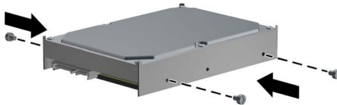
Figure 2-29 Installing Standard Guide Screws
