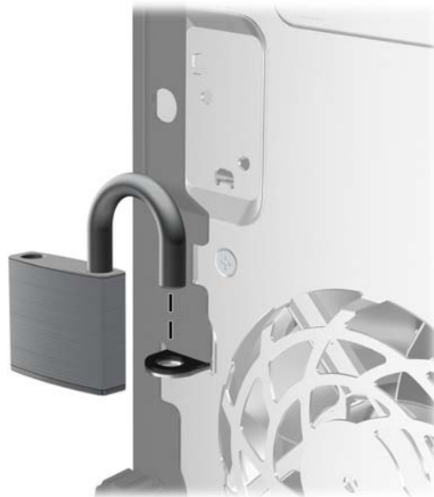
Figure 3-33 Installing a Padlock
