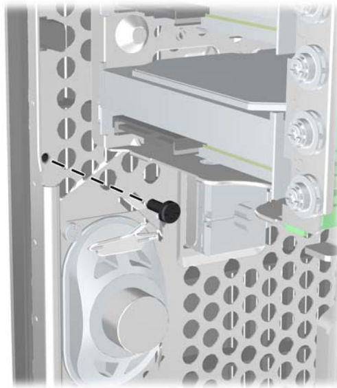
Figure 3-43 Installing the Front Bezel Security Screw
