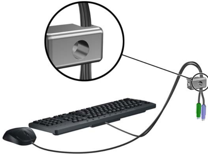
Figure 4-46 Threading the Keyboard and Mouse Cables
