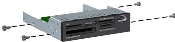
Figure 4-29 Installing Guide Screws (Media Card Reader Shown)
