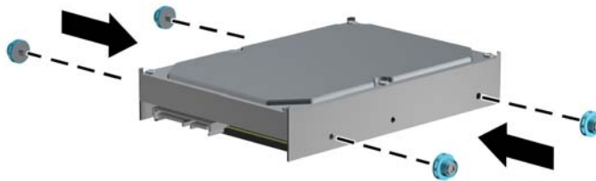
Figure 4-37 Installing Hard Drive Guide Screws
