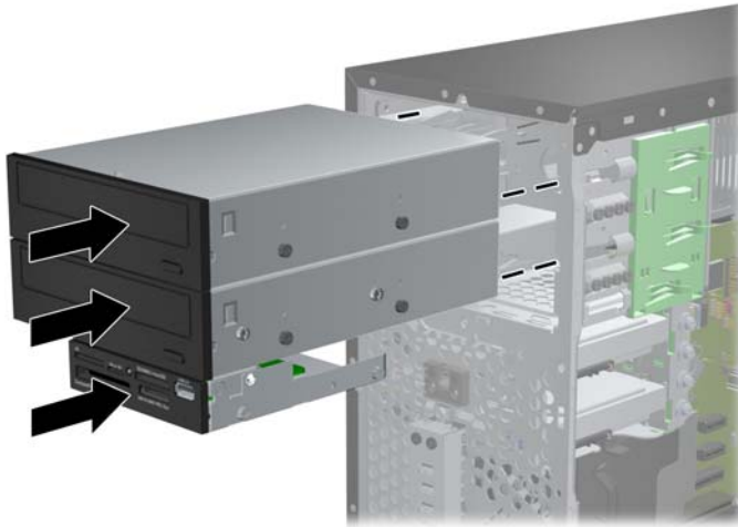
Figure 3-21 Sliding the Drives into the Drive Cage
