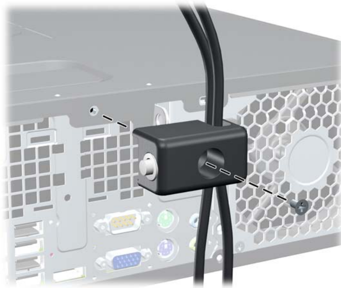
Figure 4-47 Attaching the Lock to the Chassis
