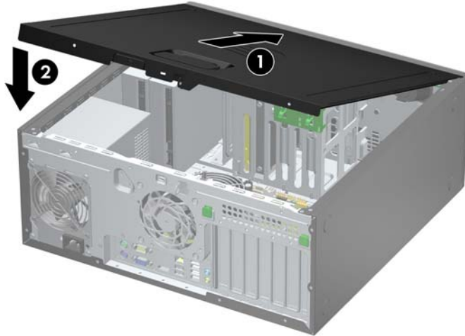
Figure 2-2 Replacing the Computer Access Panel
