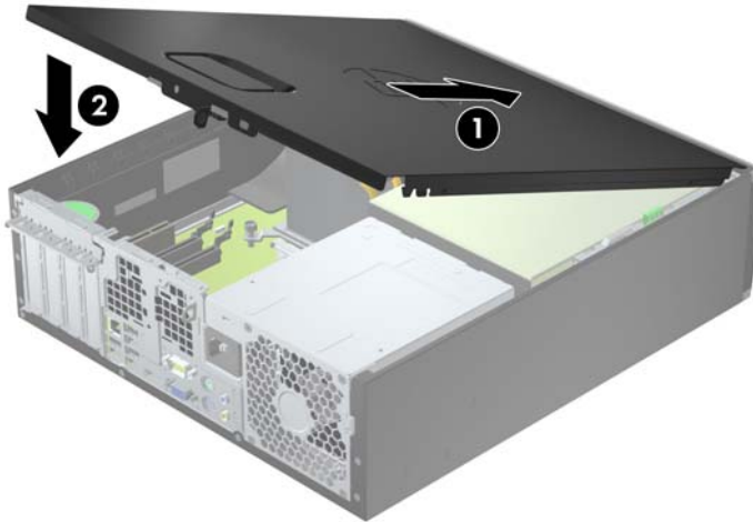
Figure 4-2 Replacing the Computer Access Panel
