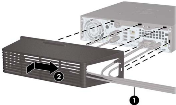
Figure 5-22 Installing a Port Cover
