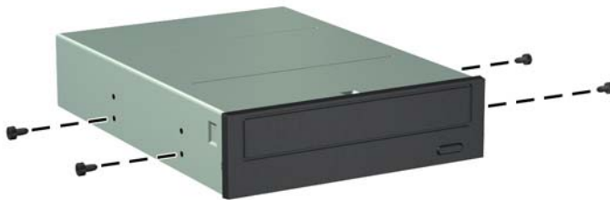
Figure 3-20 Installing Guide Screws (Optical Drive Shown)
