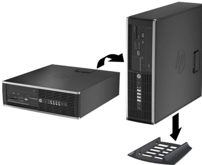
Figure 4-6 Changing from Desktop to Tower Orientation
