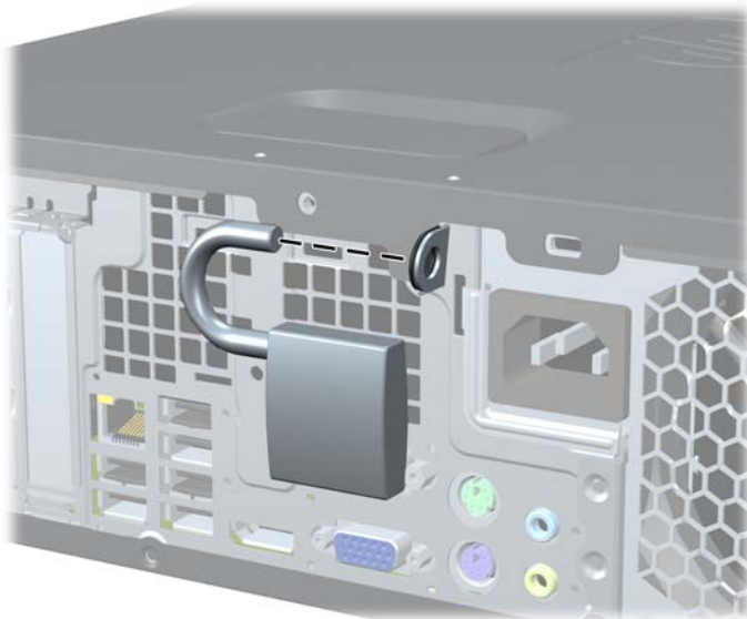
Figure 4-41 Installing a Padlock
