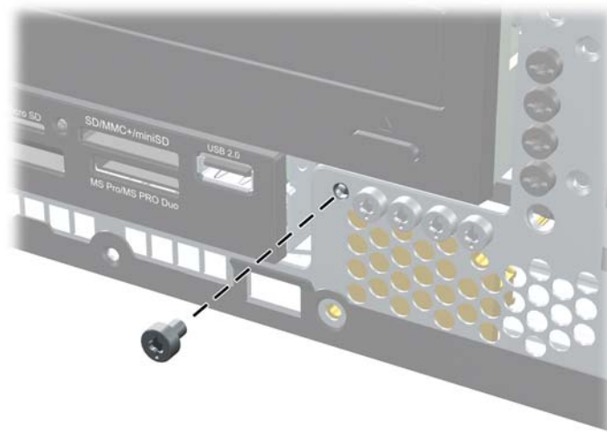
Figure 4-50 Retrieving the Front Bezel Security Screw
