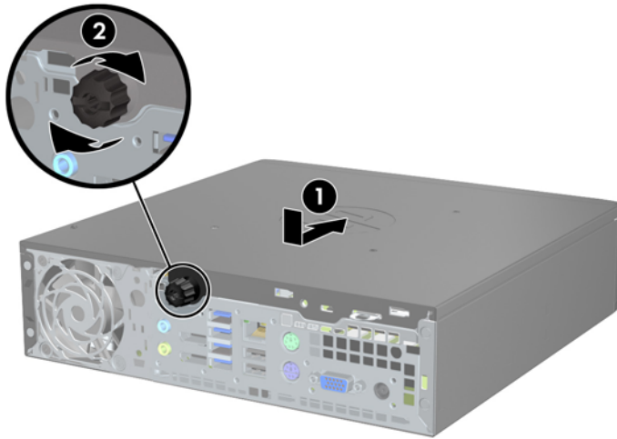
Figure 5-3 Replacing the Computer Access Panel
