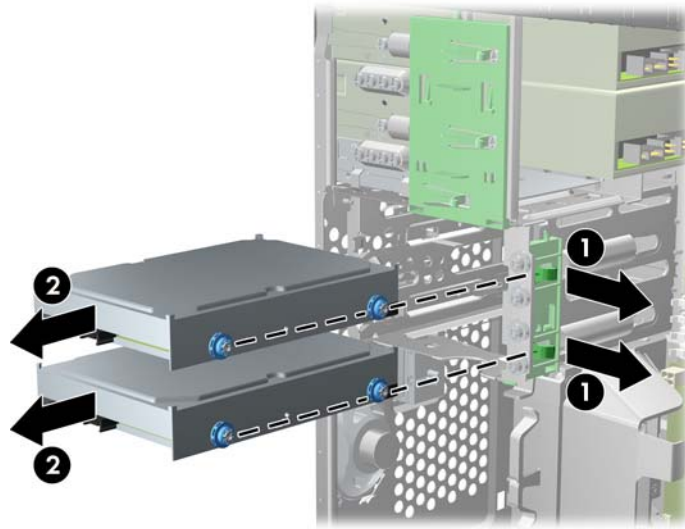
Figure 3-25 Removing a Hard Drive
