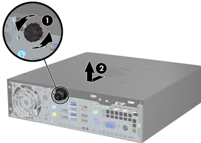
Figure 5-2 Removing the Computer Access Panel
