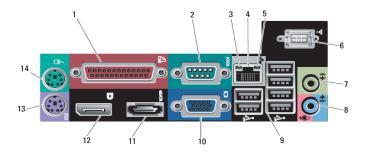
Parallel Connector 1 2 Serial Connector 3 Link Integrity Light 4 Network Adapter Connector 5 Network Activity Light 6 Wi-Fi Antenna (optional) 7 Headphone Connector 8 Line-in/Microphone Connector 9 USB 2.0 connectors (6) 10 VGA Connector 11 eSATA Connector 12 DisplayPort Connector 13 **Keyboard Connector** 14 Mouse Connector
