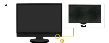
By turning part (6) in the direction shown in the figure below, the speaker turns on and the volume increases.
