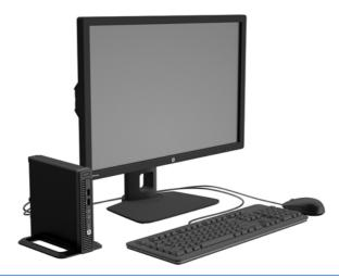
NOTE: The desktop mini can be used in a tower orientation or a desktop orientation.
