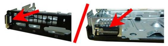
12. Remove the front transceiver from the inside of the computer by pressing the tab to disengage the transceiver and removing the transceiver (arrow in following image points to the tabs on the inside of the computer).
