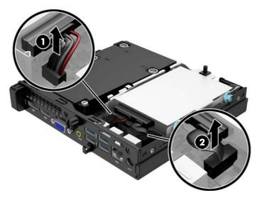
4. Pull the release lever next to the rear of the hard drive outward (1). While pulling the release lever out, slide the drive back until it stops, then lift the drive up and out of the bay (2).
