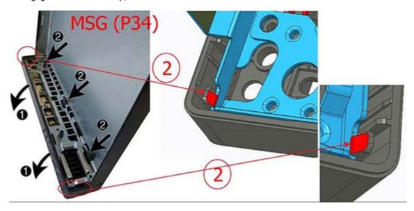
Remove the bezel from the access panel.
