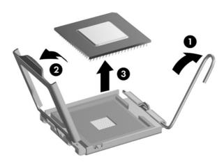
To replace the processor, reverse the removal procedures.
