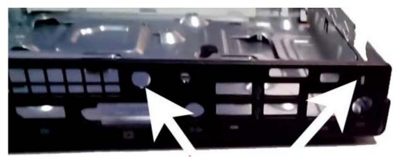
8. Insert the cable connectors into the slots on the rear of the computer, and then fasten the connectors using the included washer (on the inside of the chassis) and nut (on the outside of the chassis).
