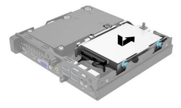
8. Connect the hard drive power cable (1) and data cable (2) to the system board.
