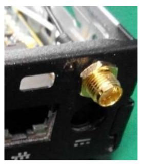
Connect the connector on the end of the black antenna cable to the connector labeled '1' on the WLAN module.
