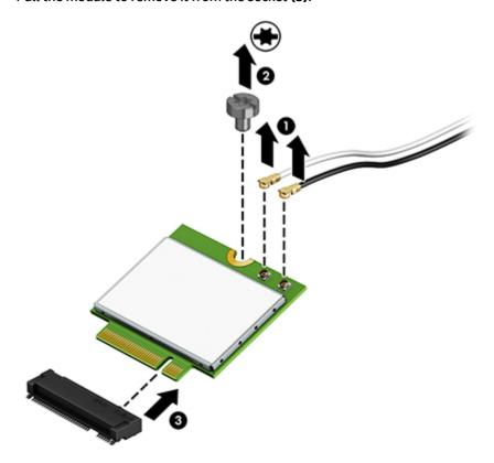
To install the WLAN module, reverse the removal procedure.
