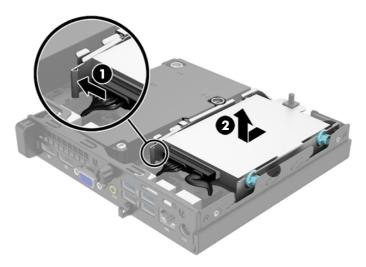
5. To install a hard drive, you must transfer the silver and blue isolation mounting guide screws from the old hard drive to the new hard drive.
