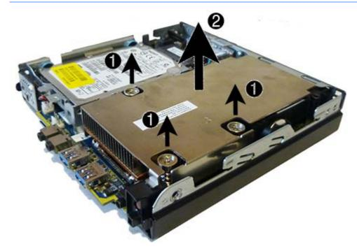
To replace the heat sink, reverse the removal procedures.
