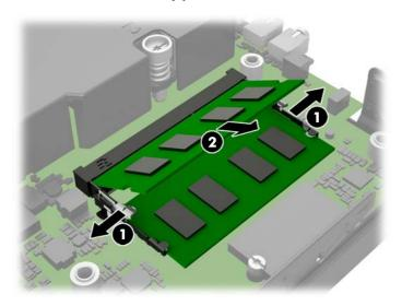
5. Slide the new SODIMM into the socket at approximately a 30° angle (1) then press the SODIMM down (2) so that the latches lock it in place.
