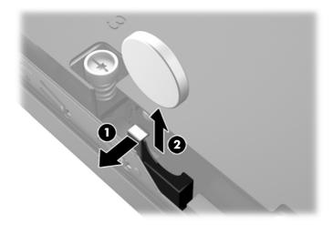
Pull back on the clip (1) and slide the replacement battery down into the holder (2). b.
