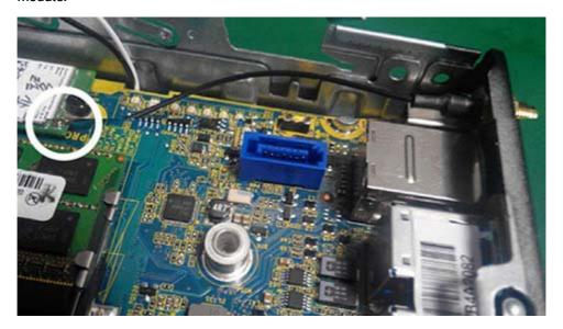
10. Route the white cable using the hooks connected to the chassis.
