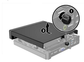
To install the access panel, reverse the removal procedure.
