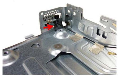
13. Remove the rear transceiver from the inside of the computer by pressing the tab to disengage the transceiver and removing the transceiver (arrow in following image points to the tabs on the inside of the computer).
