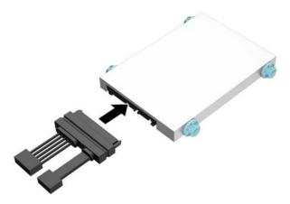
Align the guide screws with the slots on the chassis drive cage, press the hard drive down into the bay, then slide it forward until it stops and locks in place.
