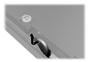
**b.** Lower the battery so that is next to the holder then push it into the holder.
