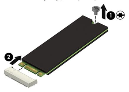
To install the M.2 SSD, reverse the removal procedures.
